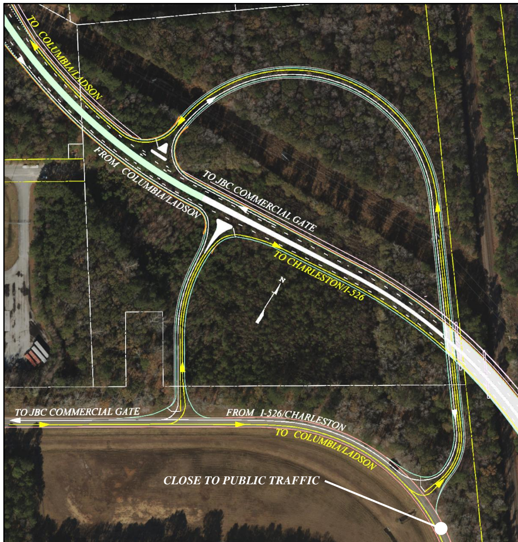
Figure 5. Proposed Access to/from JBC Commercial Gate from PCP3
